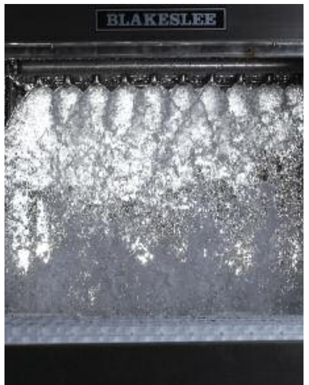
Top and bottom mounted water jets provide torrential cleaning & rinse action.
